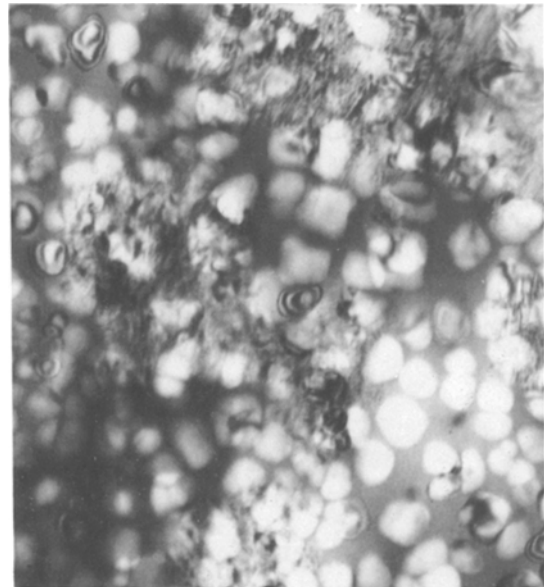
Figure 5 Typical microstructure obtained during the MS-II reaction after 95 sec at 550 K: striated grains are observed to consume the uncrystallized amorphous material ( \times 59\,000 ).
